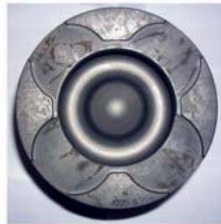
S6D140 6212-31-2151 Total Height 125.2mm, Combustion Chamber 78mm
